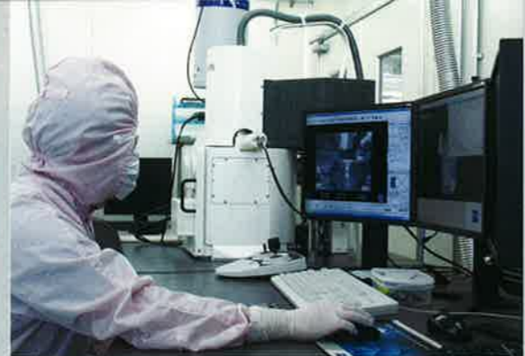
走査電子顕微鏡/X線分析装置 (FE-SEM/EDX) Field emission scanning electron microscopy/Energy dispersive x-ray analyzer (FE-SEM/EDX)
