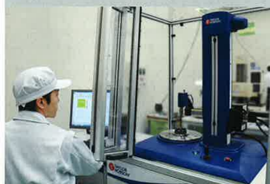
高精度真円・円筒測定機/軸受評価・解析 High-precision Circularity Measuring/bearing components evaluation・Analysis
