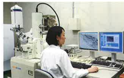
5~10万倍の表面観察/元素分析・定量分析 Surface observation (50,000-100,000 times magnification) / elemental analysis and quantitative analysis
